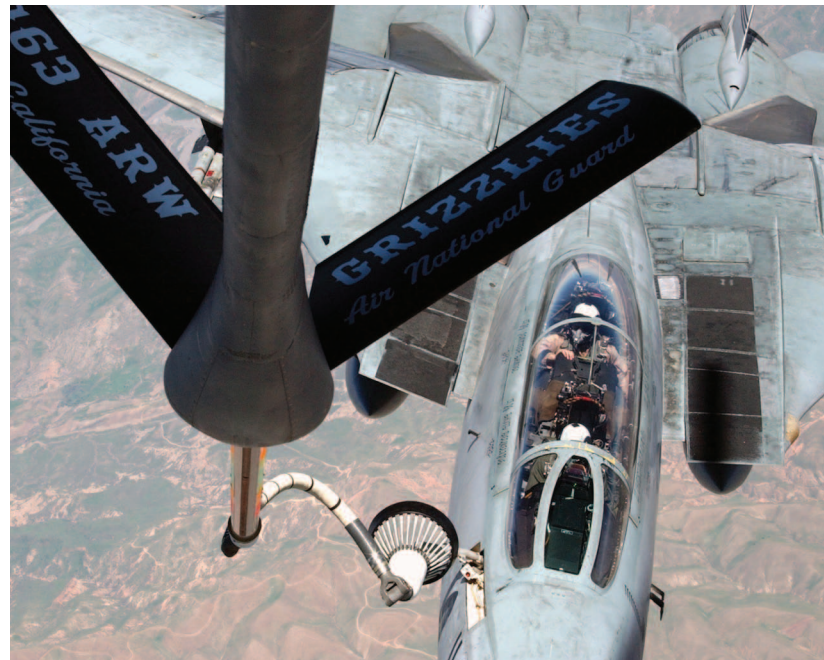
A U.S. Navy Grumman F-14 Tomcat receives fuel from an Air National Guard Boeing KC-135 Stratotanker during a combat mission. (U.S. Navy photo by Paul Farley)
