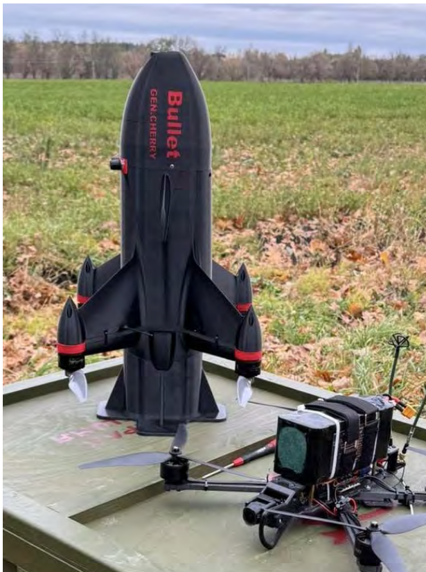
A General Cherry Bullet interceptor designed to down Iranian Shahed and Russian Geran-2 drones. Photo credit: General Cherry.
